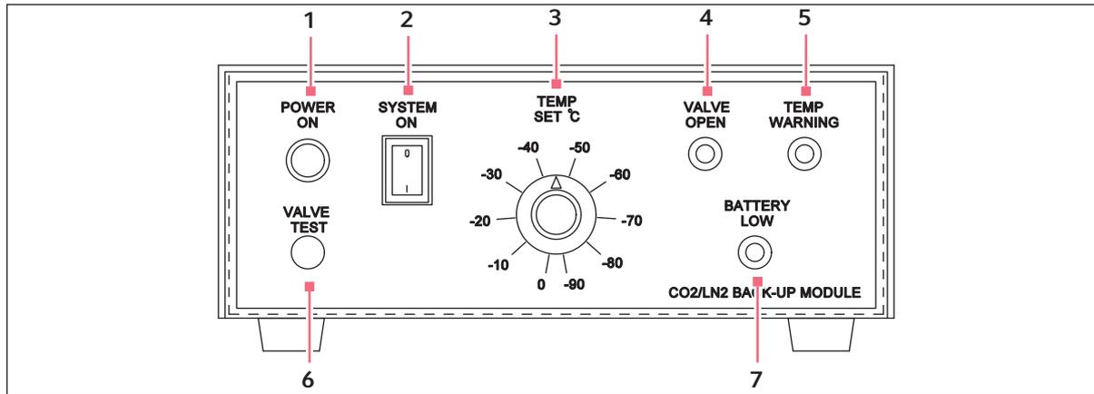
Fig. 3-1: Front view of the LN<sub>2</sub> Back-up System
