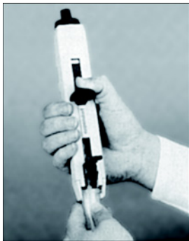
Fig. 3: Inserting the Varitip
