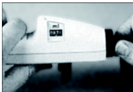
Fig. 5: Setting the volume
